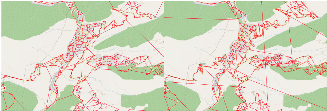
Figure 4.3: Hilbert-Order on the left side vs. Z-Order on the right side. The line between nodes shows their order. I.e. node 1 is connected to node 2, which is connected to node 3, ... Hilbert-Order seems to have fewer big jumps, suggesting better locality.
